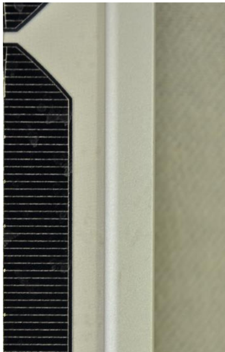
Fig. 6: detailed left side view to frame after ammonia corrosion test
